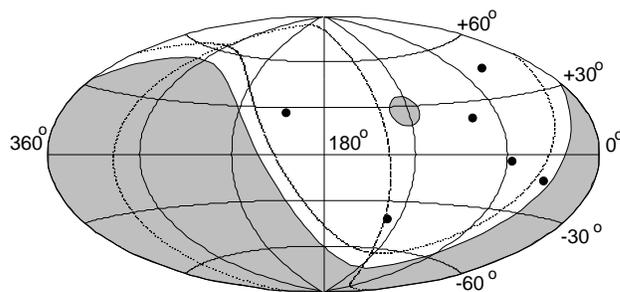
FIG. 3. Arrival directions of six  $10^{20} \text{ eV}$  events on the Galactic coordinates. The shaded regions indicate the nonobservable celestial regions due to the zenith angle cut of  $\leq 45^\circ$ . The equatorial and supergalactic planes are also shown.
